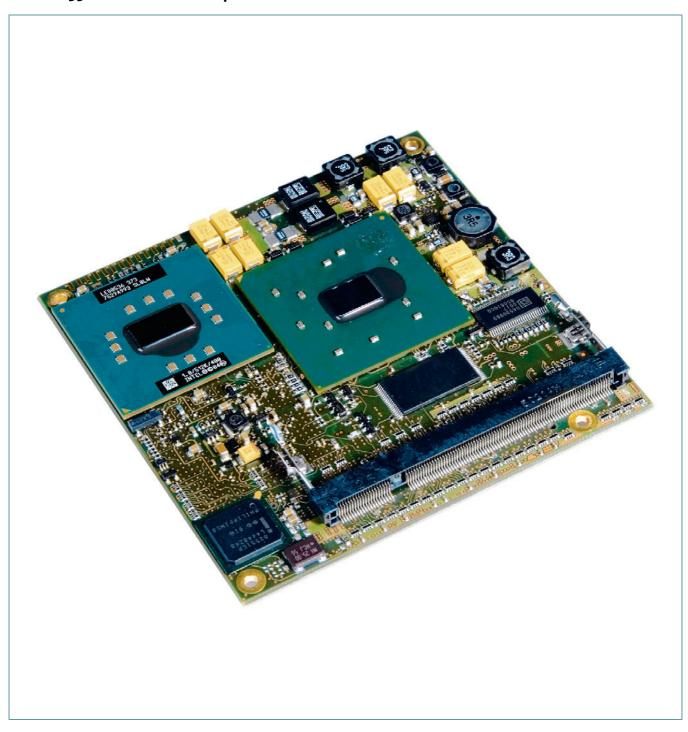
COM Express, an open specification of the PICMG (PCI Industrial Computer Manufacturer Group), is a module concept to bring PCI Express and other latest technologies like SATA, USB 2.0 and LVDS on a COM (Computer On Module). COM Express is plugged onto an application-specific base board similar in the ETX concept, but offers more options and a growth path to future CPU technologies. Utilizing different sizes, COM Express can be used for highly embedded solutions up to high performance platforms.
