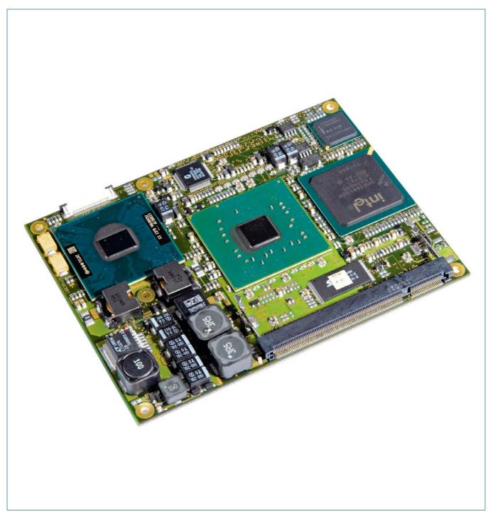
COM Express, an open specification of the PICMG (PCI Industrial Computer Manufacturer Group), is a module concept to bring PCI Express and other latest technologies like SATA, USB 2.0 and LVDS on a COM (Computer On Module).
