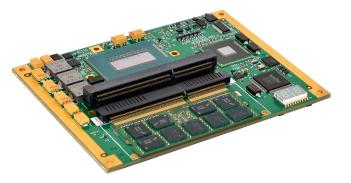
The XCOM-6400 CPU processor module has Type 6 interconnects and features the 4<sup>th</sup> generation "Haswell" Intel processor. The Core i5 allows for lower power consumption (around 20-40%), while the Core i7 provides higher performance- as much as twice the performance of "Sandy Bridge" (3<sup>rd</sup> generation).
