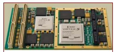
Acromag FPGA PMC card enables reconfigurable high performance I/O processing and user-customizable computing for video, 3D data, radar/sonar, software-defined radio, electronic warfare, floating-point math and fuzzy logic algorithm applications.
